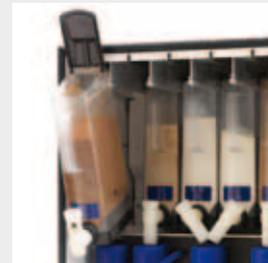
*The ingredient containers have a handle, so they are easy to pull out and re-fill. The lid opens automatically and the containers can be filled quickly and easily, either in or out of the machine.*
